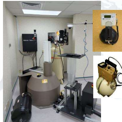
Neutron irradiator with a 3 Ci AmBe source (2 reference detectors)
