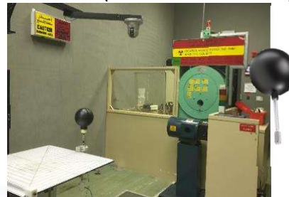
Gamma irradiators with 06 ^{137}\text{Cs} and 01 ^{60}\text{Co} sources (two reference chambers)
