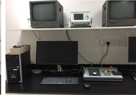
Control room of X-ray Irradiator (Narrow Beam)
