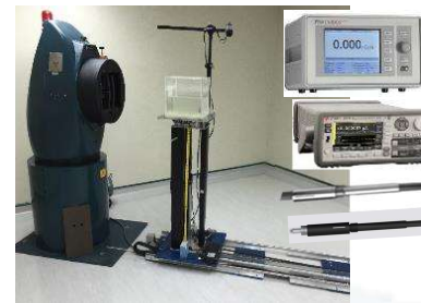
Brachytherapy unit ^{192}\text{Ir} source (01 ref. chambers and 01 electrom.)
