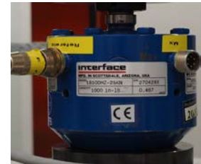
Strain gauge force transducer – C_{DMS}
