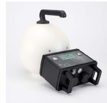
Linearity test of a NMS017 survey meter Courtesy from Neil Roberts - NPL
