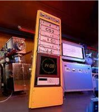
Cs atomic beam frequency standard (PTB)
