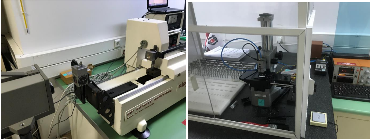
(Fig.6 )onsite calibration for short gauge blocks comparator and length measuring machine.
