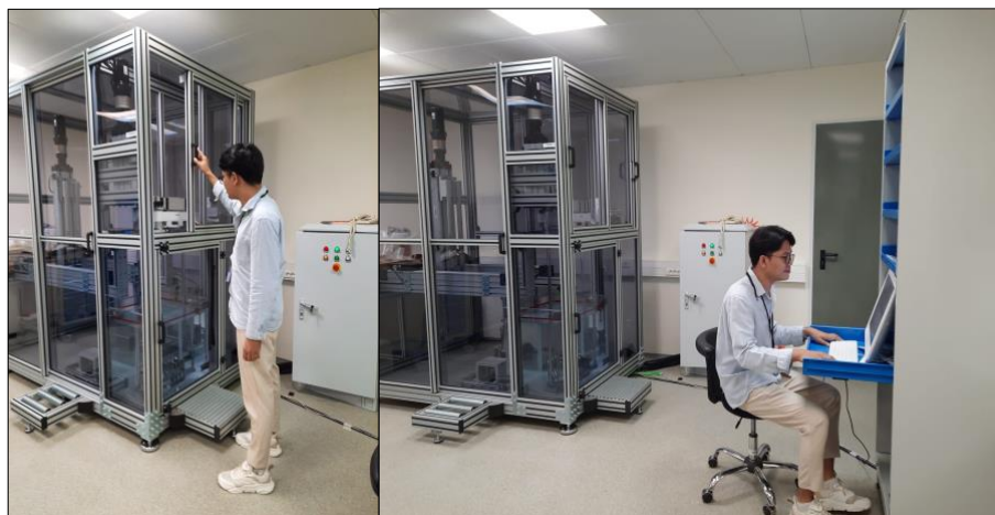
Figure 1: The trainee operating the high-capacity measure volume and density measurement system of TUBITAK-UME
