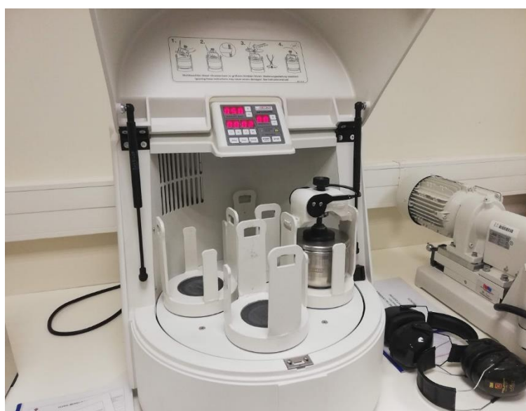
Figure 2 - Ball milling system
