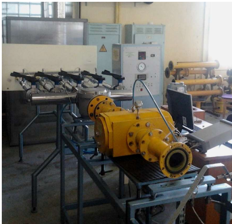
Figure 10 – Test bench in LEI with sonic nozzles
