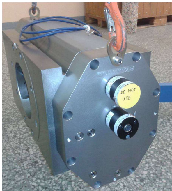
Figure 2 – Pulse connector of rotary piston gas meter ELSTER-INSTROMET IRM-3-DUO G650
