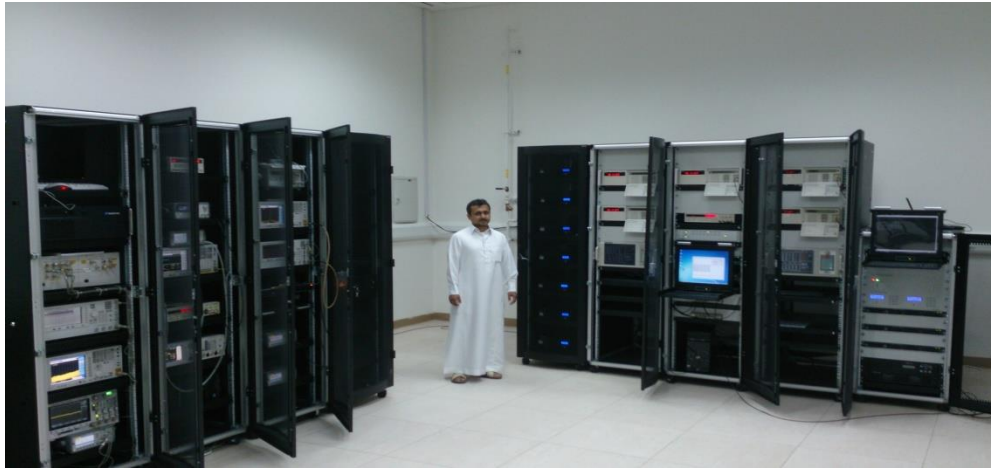
Figure 2. Photograph of SASO time and frequency system
