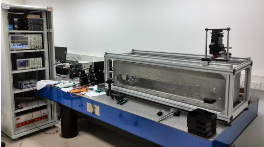
Laser Homodyne Calibration System
