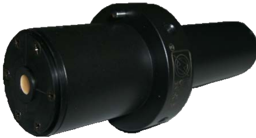
Luminous flux standard LED for high-power LED Calibration (luminous flux is about 60 lm)
