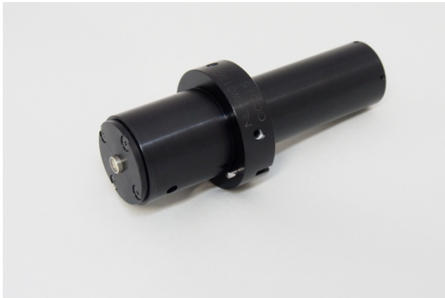
Standard LED for Luminous Flux Calibration (luminous flux is about 1.3 lm)
