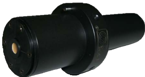
Luminous flux standard LED for high-power LED Calibration (rated luminous flux: 68 lm)
