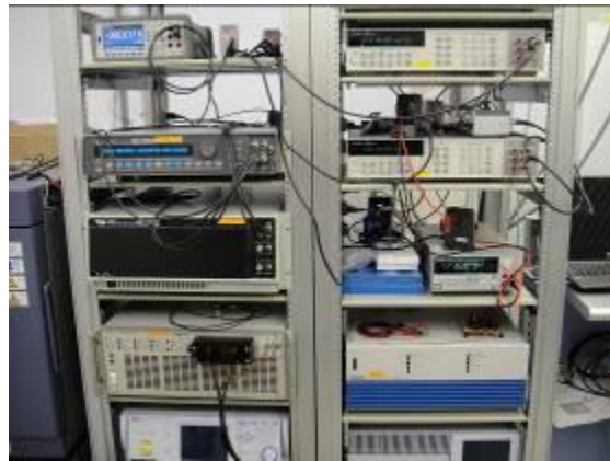
Fig. 1 Photograph of the electrochemical impedance measurement system developed using the Frequency Response Analyzer and the Potentio-Galvano Stat.
