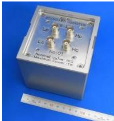
Fig. 1. Photograph of the developed 1-kΩ metal-foil resistor
