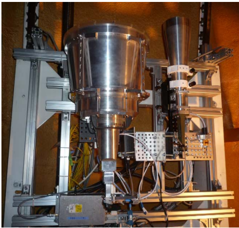
Fig. 12. Picture of the broadband feed mounted on NICT Kashima 34m radio telescope. The first prototype broadband feed (IGUANA-H for 6.5-15GHz) in the right and the second prototype (NINJA for 3.5-14GHz) in the left.
