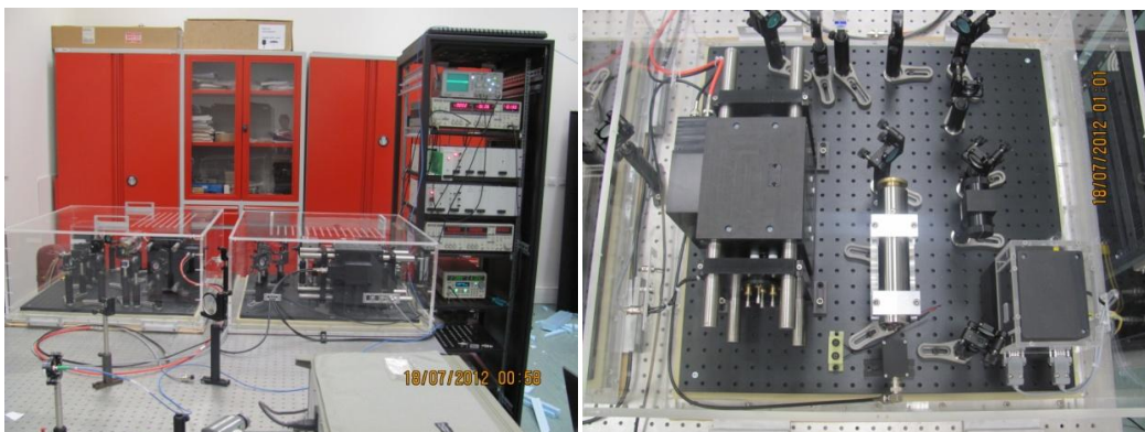
2 ECDL laser systems stabilised on S-D two-photon transition of Rb atoms
