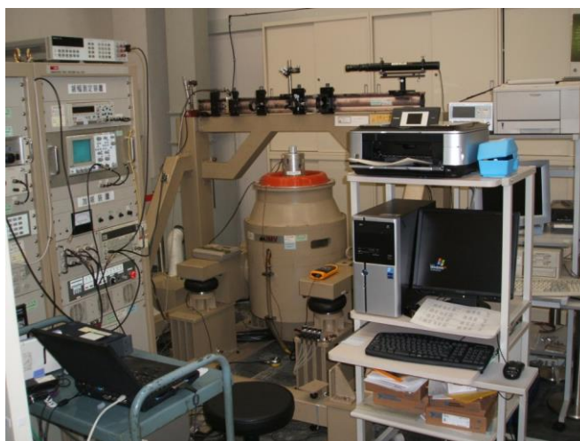
Fig. V2 System 2: Low-frequency vibration calibration system (CMC not published yet for 1 Hz to 40 Hz)
