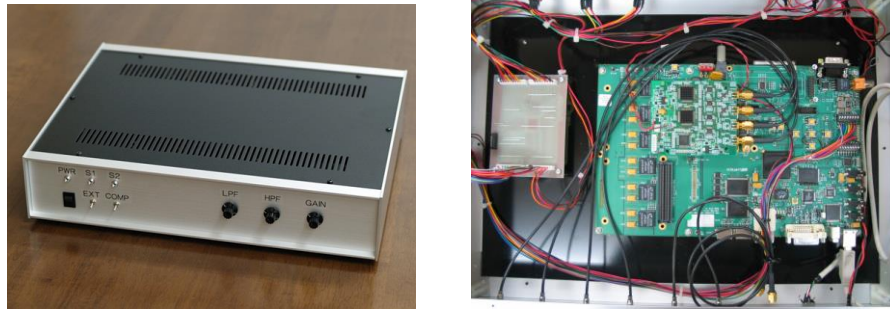
Fig. V8 Digital demodulator for laser vibrometer standard
