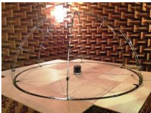
Fig. A1: Hemisphere frame for fixing microphones and RSS located in anechoic chamber
