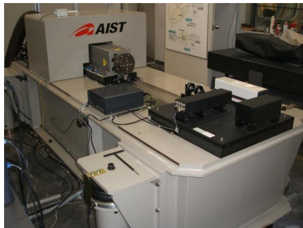
Fig. V1 System 1: Very low-frequency vibration calibration system
