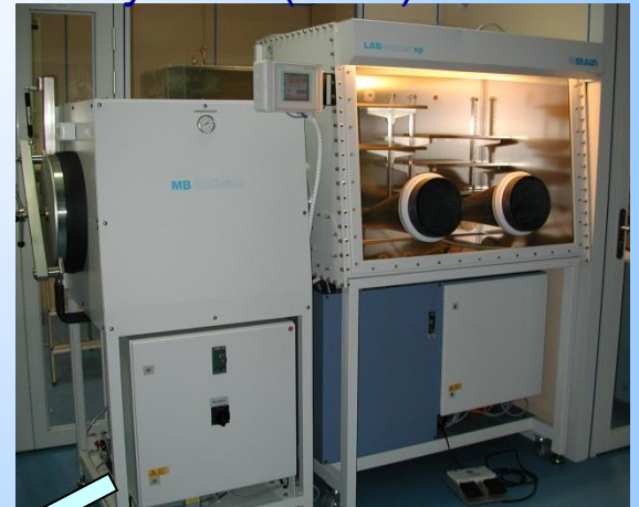
Vacuum Transfer System (VTS)
