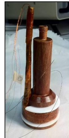
The Cryogenic Current Comparator Amplification and its shield
