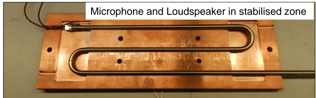
calibration zone with Peltiers
