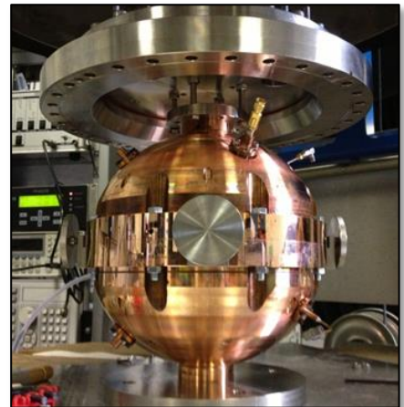
misaligned 3-litre copper sphere
