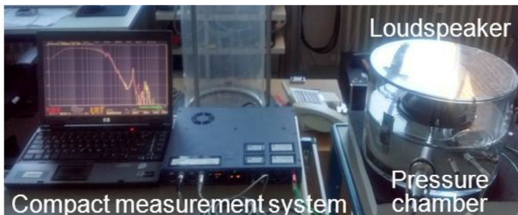
Fig 7 - Inmetro's setup used for calibration by simultaneous comparison of a microphone with its vent exposed to the sound field
