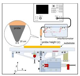
In framework of PlanarCal project (14IND02), VSL extended low-noise S-parameter measurements to highly mismatched nano-scale devices. VSL and Delft University of Technology have developed a broadband interferometer-based VNA measurement system suitable for highly mismatched measurements.
