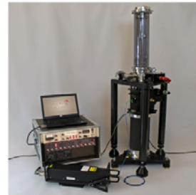
Figure 2. Gravity measurements in the WB laboratory. The 3 AGs occupied W1 and W2 and the 8 RGs measured the ties between W1 and W2 at the five levels and the 3D grid around the WB.
