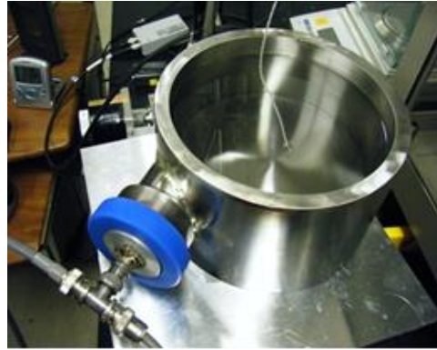
Water bath for calorimetry
