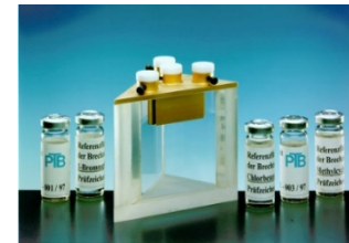
Minimum deviation angle method
