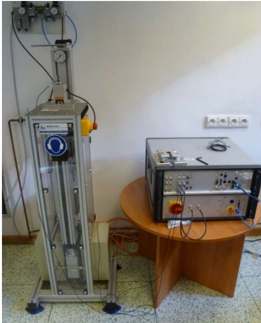
Fig. 2 CS18 LMS measuring set-up for secondary shock calibration
