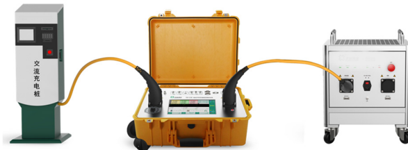
Figure 1. Fielding Calibrating of EV Charging Spot with virtual load facilities
