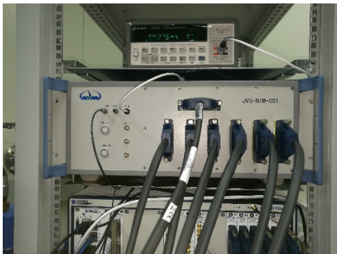
Fig. 2. PJVS drive system
