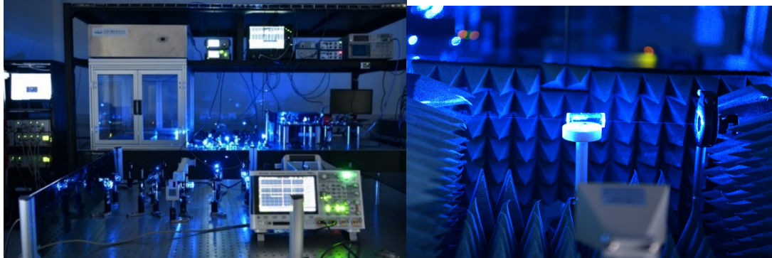
a) Experimental Setup; b) The room-temperature atomic vapor cell is used as a quantum probe for detecting RF E-field.
