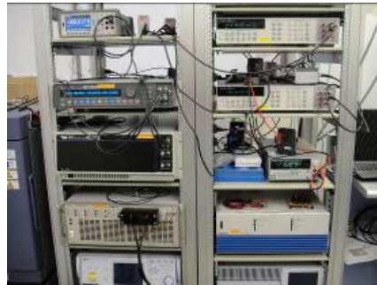
Fig. 7 Photograph of the electrochemical impedance measurement system developed using the Frequency Response Analyzer and the Potentio-Galvano Stat.
