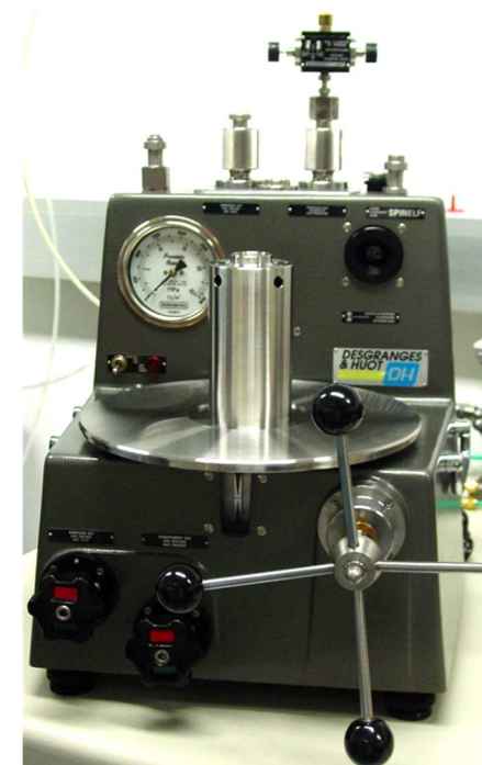
Gauge Pressure Balance – Gas Medium 40 kPa to 2 MPa CMC: 1.2 Pa to 60 Pa
