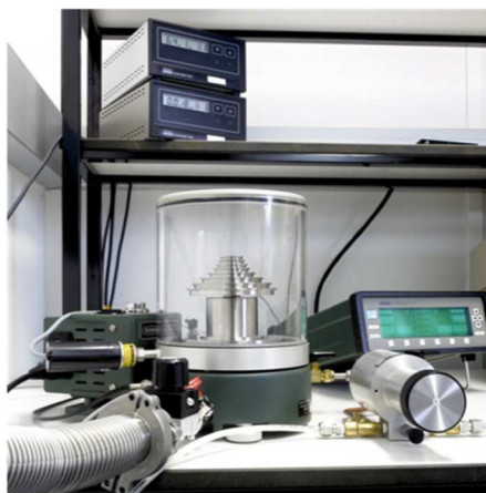
Gauge/Absolute - Pressure Balance 3.5 kPa to 170 kPa CMC: 0.52 Pa to 6.4 Pa (Absolute) 0.11 Pa to 5.1 Pa (Gauge)
