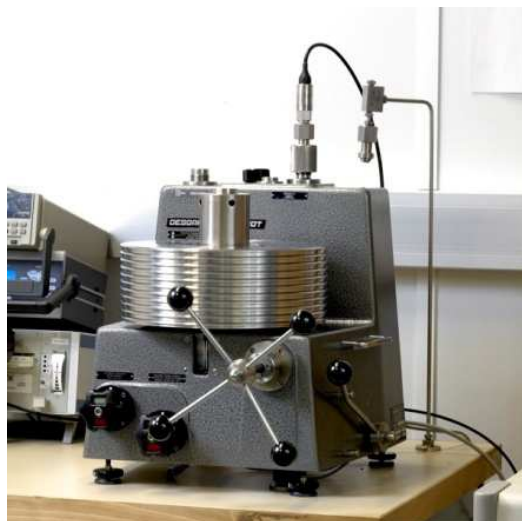
Gauge Pressure Balance – Oil Medium 0.2 MPa to 100 MPa CMC: 29 Pa to 5.5 kPa
