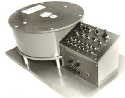
Compensated current comparator KPK2 (5 – 1 200) A/5 A, uncertainty 10 ppm
