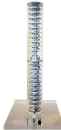
AC/DC voltage divider up to 20 kV standard uncertainty 40 ppm
