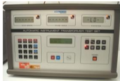
Transformer test set Tettex 2767
