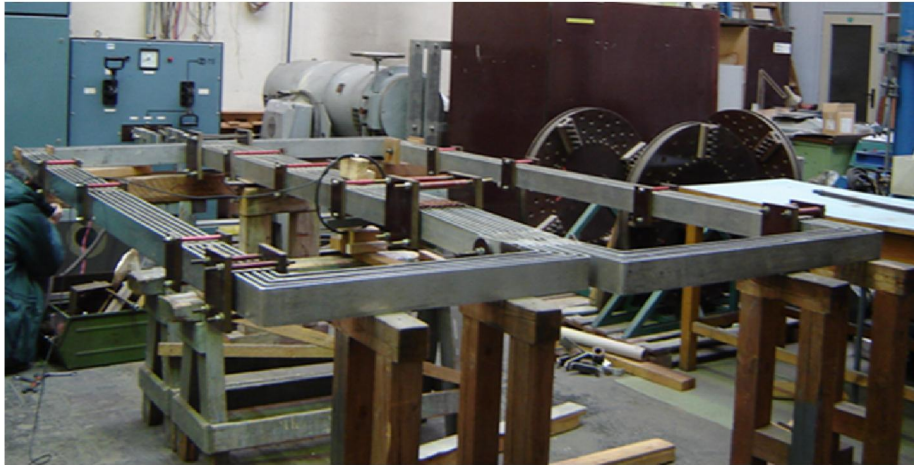
Current loop for AC current meter testing up to 30 kA
