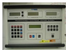
Electronic voltage burden Tettex 3695
