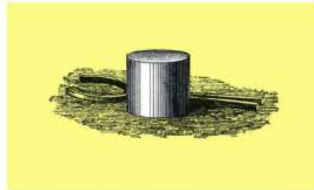
A 19th-century illustration of the International Prototype Kilogram (IPK), the original standard kilogram
