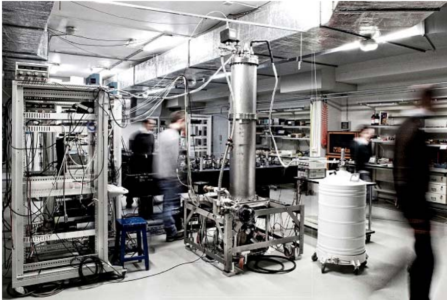
Figure 3: The cryogenic fountain IT-CsF2
