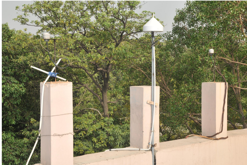
Fig. 9: GPS antenna unit of TTS2 receiver and Septentrio receiver system installed
