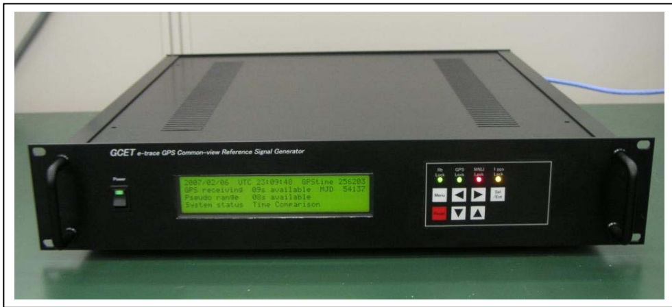
Fig. 7. Terminal equipment of frequency remote calibration service.
