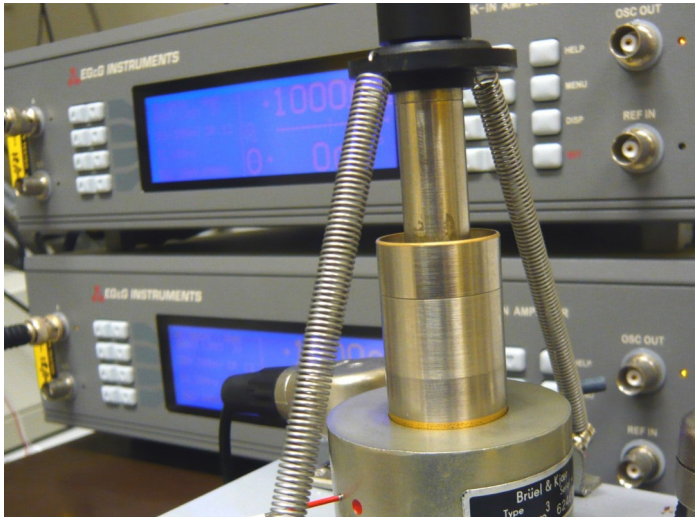
Figure 4.1: The NPL reciprocity equipment shown here being used to calibrate LS1P microphones, which are the subject of the proposed CCAUV.A-K5.
