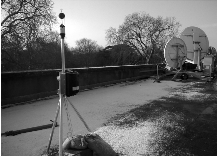
Figure 4.3: A DREAMsys unit under test at NPL, illustrating the resilience of the system to harsh weather conditions.
