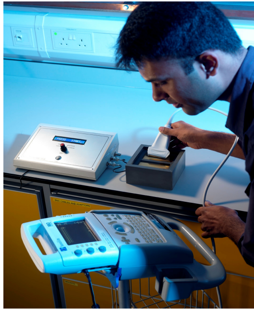
Figure 6.5: Image of the prototype NPL Ultrasound Pyrometer developed to determine the acoustic power generated by medical diagnostic equipment.
