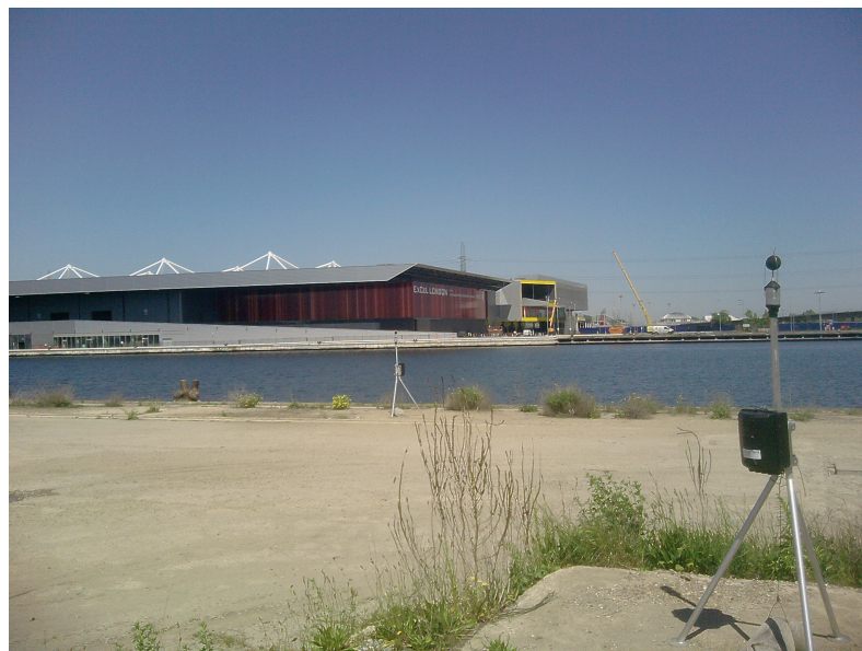
Figure 4.4: Two of the forty DREAMSys units deployed at the site adjacent to London City Airport. The units monitored noise continually for a six month period, reporting data wirelessly.
