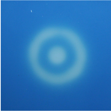
Figure 6.3: Photographic images derived using the Thermochromic tile developed at NPL, using a transducer operating at 3 MHz, and nominal intensity setting 1 \text{ W cm}^{-2} for a time exposure (reading from top to bottom) of 10s, 7s and 5s. The x -axis is in mm and the y -axis is in arbitrary units.
