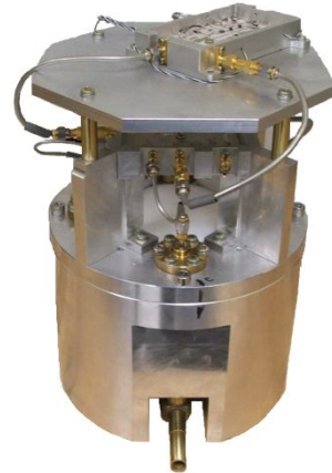
Figure 17. Traveling wave WGR oscillator construction.
