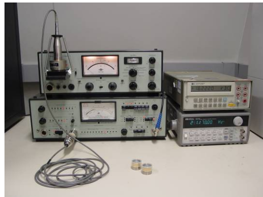
Fig. 6: System for calibration of 1'' microphones by comparison in pressure-field
