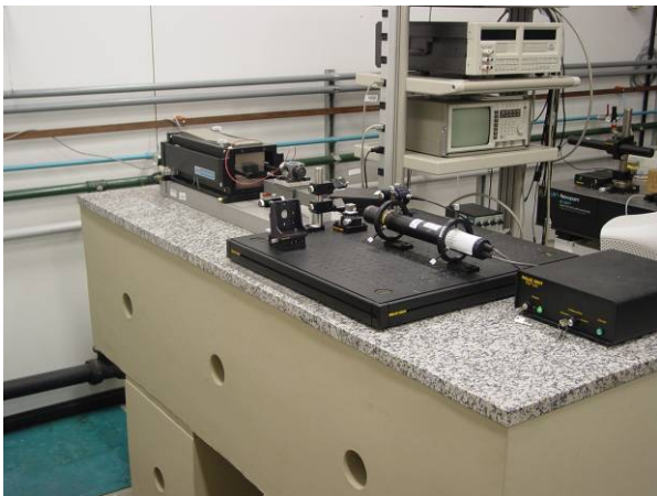
Fig. 8: Low-frequency absolute calibration system of accelerometers
