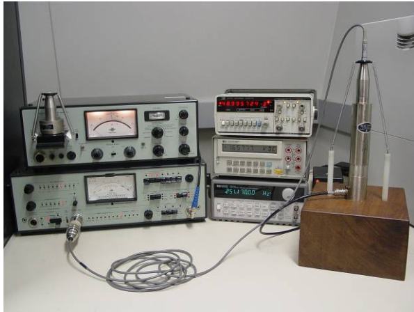
Fig. 3: System for calibration of pistonphones by the insert voltage technique
