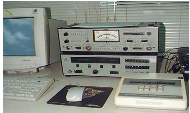
Fig. 4: System for calibration of sound level meter calibrators
