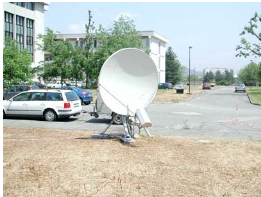
Figure 6. The TUG portable station collocated at IEN during the IEN-PTB link calibration activity
