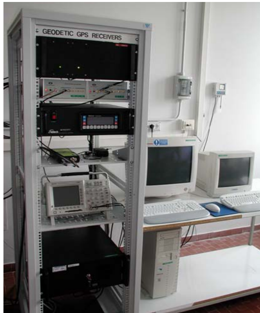
Figure 5. The geodetic receiver set-up
