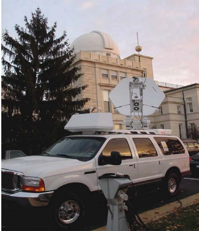
Figure 10. Mobile Earth Station for TWSTT calibration has been driven 18,000 miles this year. Small enough to be carried on a C141 military transport plane, it could be equipped to serve as a hop-link by communicating through two different satellites and/or frequencies simultaneously. Its automated pointing system makes it easy to find a satellite in the field. In the background one can see a functional copy of the Time Ball originally built to transfer time to ships sailing up the Potomac River.
