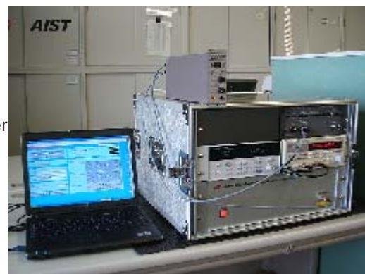
Calibration system for charge amplifier
