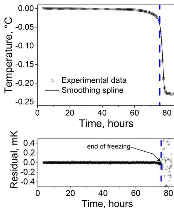
**Figure 12.** Illustration of the spline method for determining the end-point of a freeze. The appearance of ‘noise’ (i.e. residuals in the spline fits) suggests that the endpoint is at about 76.4 h. [Pearce *et al.* (2013)]<sup>4</sup>. Note that the end-point of freezing occurs at a temperature way below the plateau (this is also the case for the heater power determination of the end-point in Figure 11).
