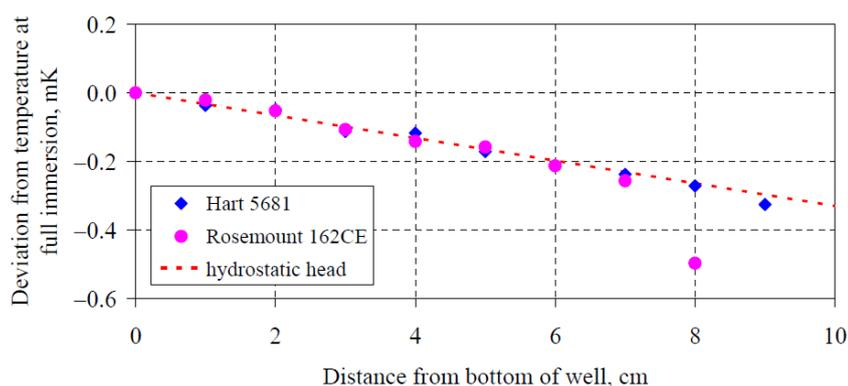
**Figure 9.** Immersion profile during realization of In freezing point [Strouse (2008)]<sup>3</sup>.
