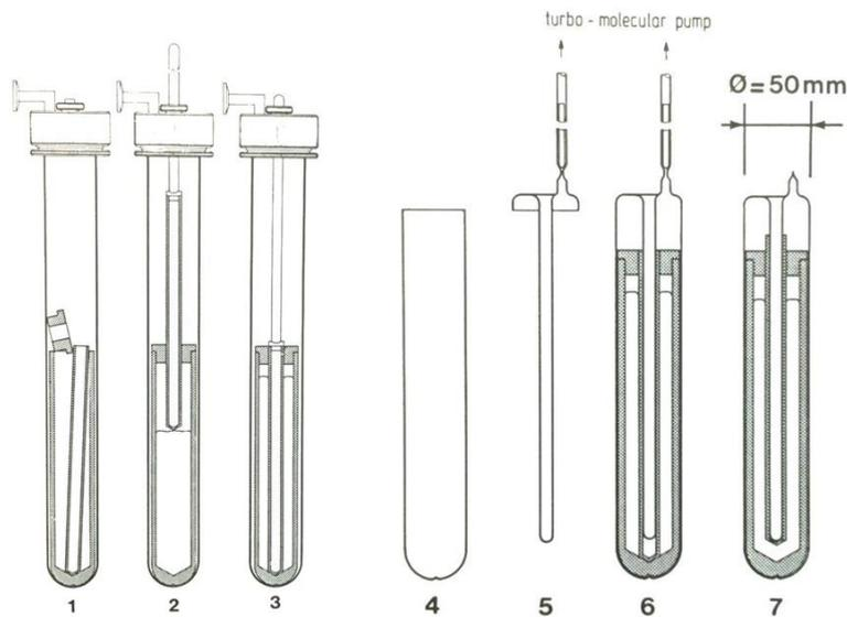
**Figure 4.** Preparation and filling of a sealed cell suitable for the freezing points of In, Sn, Zn, Al, and Ag [Nubbemeyer (1990)]: (1) Parts ready for baking in vacuum. (2) Join the graphite parts and the metal block (or shot) of the fixed-point cell. (3) Melt the metal block and lower the graphite well completely. (4) and (5) Quartz parts ready for degreasing. (6) Assemble crucible and quartz parts, seal the quartz, evacuate and fill with argon. (7) Seal off.
