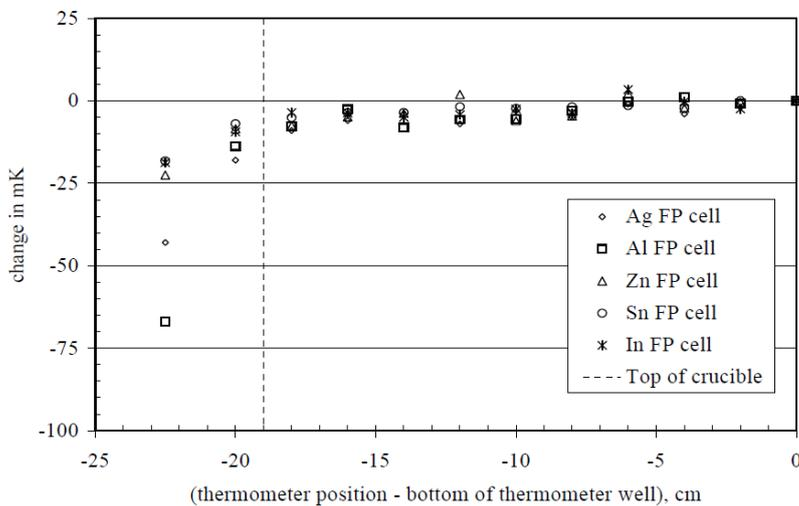
**Figure 8.** Vertical temperature profiles for several fixed-point cells, with furnace temperature 2.5 °C below the freezing point of the fixed-point cell. The thermometer position is relative to full insertion in the well [Strouse (2008)]<sup>2</sup>.
