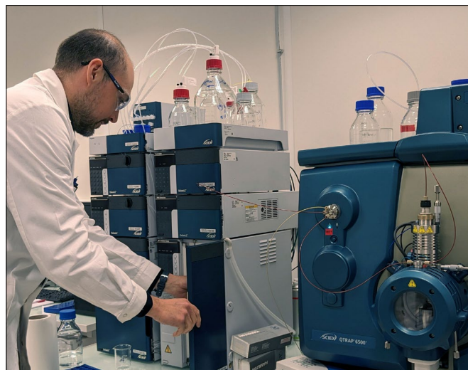
LC-MS/MS instrument used for CCQM peptide and protein comparison sample characterization
