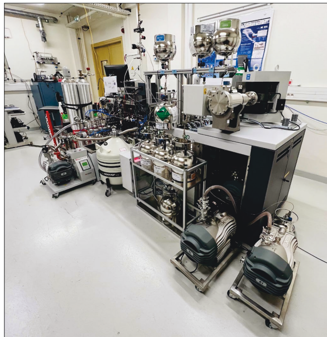
Isotope ratio mass spectrometer for \delta^{13}\text{C} and \delta^{18}\text{O} measurements in CO 2 in air standards with cryogenic extraction system
