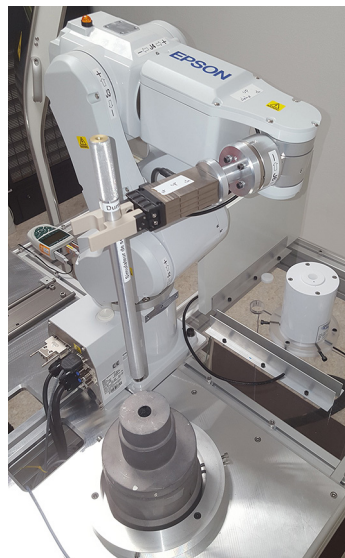
The new BIPM facility for the BIPM.RI(II)-K8 comparison. The image shows manipulation of a radioactive source using a robotic arm to study the stability of the brachytherapy standard
