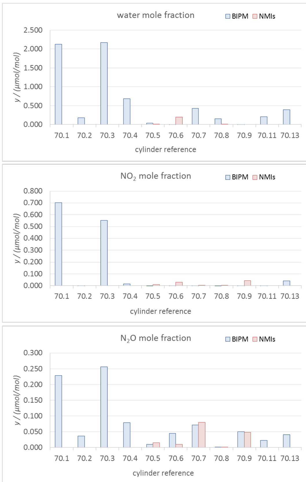
Figure 5: Mole fraction of H 2 O, NO 2 and N 2 O in standards prepared at 70 μmol mol -1 , as measured by FTIR at the BIPM (blue bars) and as reported by participants (pink bars). Absence of a bar indicates that the participant did not report any value.
