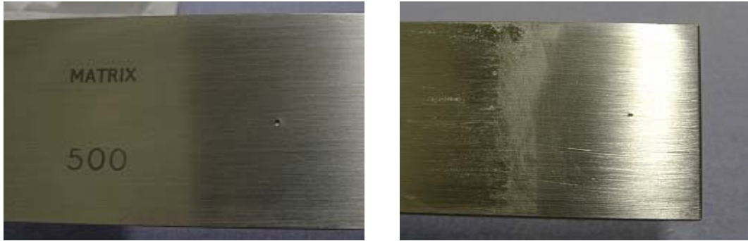
Figure 3 Side face damage to the 500 mm gauge blocks in the first loop, as photographed by pilot laboratory at end of loop 1.
