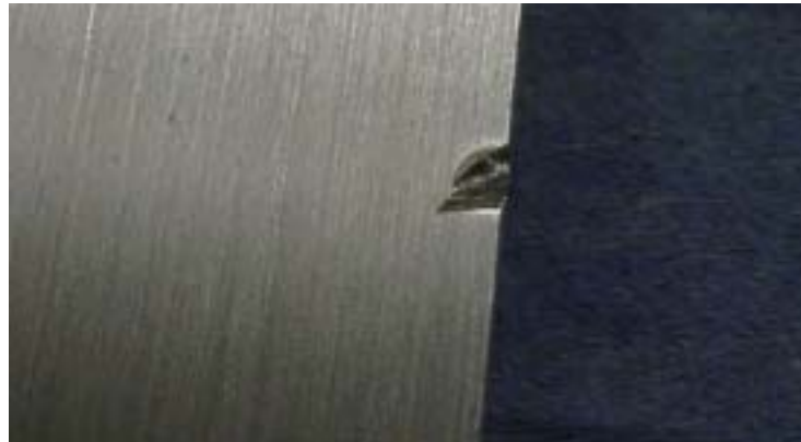
Figure 4 'Hack' mark on the side face of the 500 mm gauge block S/N AA/71001 (loop 2)
