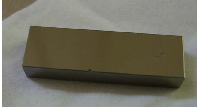
Figure 3 - damage to the 5 mm tungsten carbide gauge block
