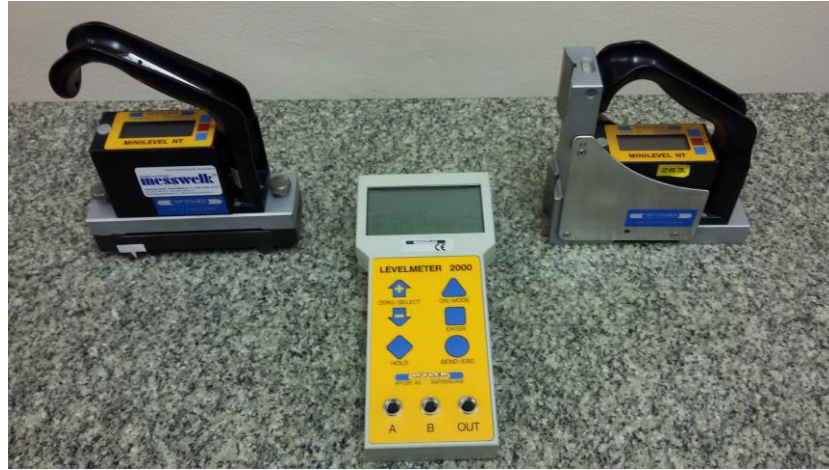
Figure 4 – Overall view of the measurement system “Electronic level meter WYLER” maintained at BelGIM
