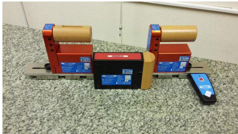
Figure 5 – Overall view of the measurement system “Electronic level meter WYLER” maintained at UNIIM
