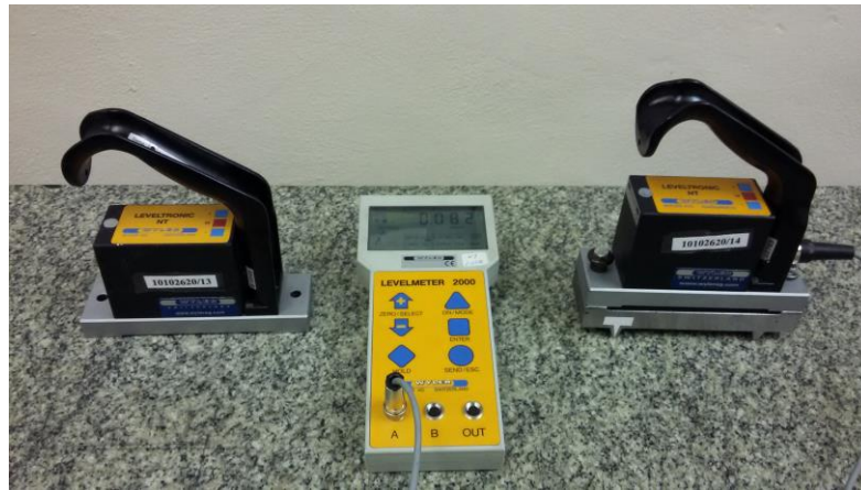
Figure 6 – Overall view of the measurement system “Electronic level meter WYLER” maintained at SKS RSE KazInMetr
