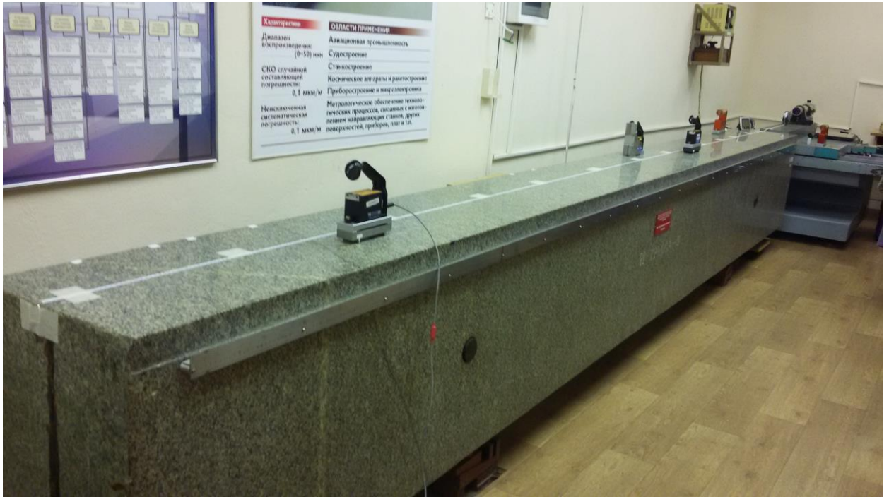
Figure 2 – Transfer Standard (UNIIM special solid-stone bridge)
