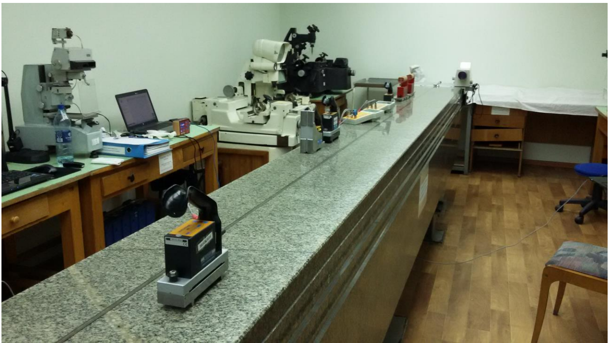
Figure 3 – Transfer Standard (SKS RSE KazInMetr special solid-stone bridge)
