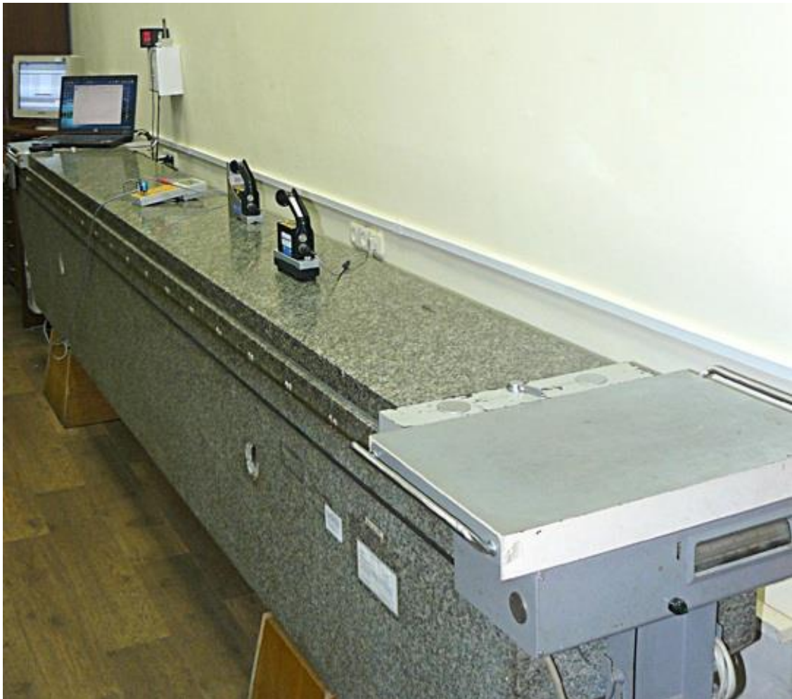
Figure 1 – Transfer Standard (BelGIM special solid-stone bridge)
