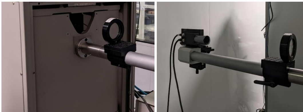
Figure A1. Modification to imaging arm of the VTT MIKES phase stepping gauge block interferometer.
