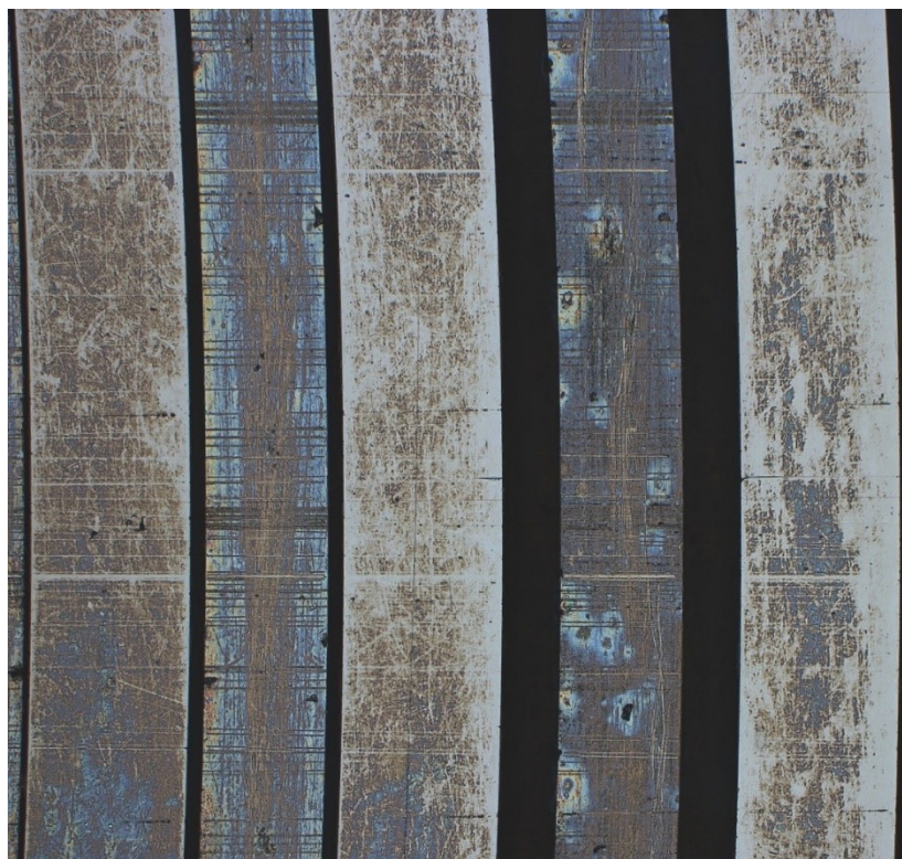
Figure 23 Microscope DIC image of artefact EN19_7 showing the huge number of scratches produced by tactile measurements.
