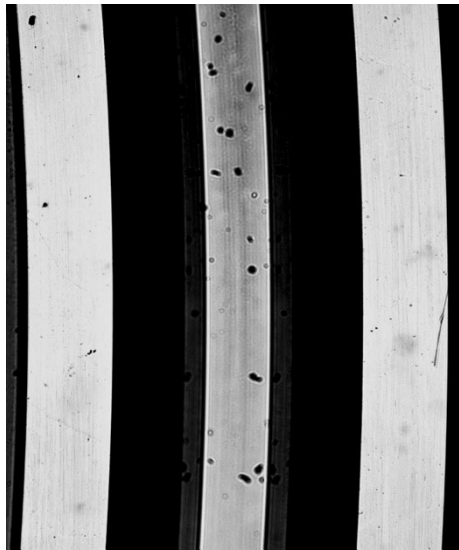
Figure 15 Microscope image of 600 \mu\text{m} groove before comparison measurements
