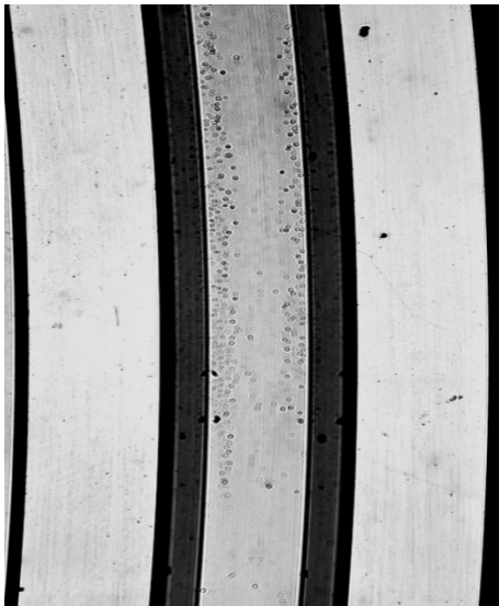
Figure 13 Microscope image of 200 \mu\text{m} groove before comparison measurements
