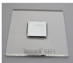
Figure 31 The SiMetrics depth setting standards consist of a glass plate with the bonded silicon chip on it and an engraved serial number
