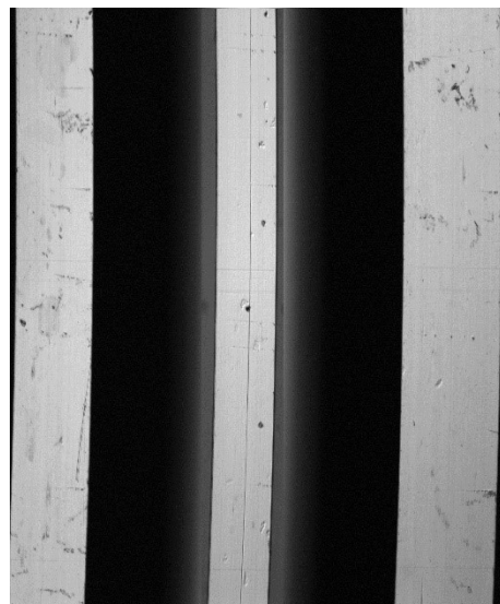
Figure 16 Microscope image of 600 \mu\text{m} groove after comparison measurements
