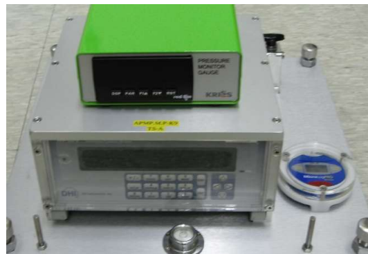
(b) Modified transfer standard with a monitor gauge
