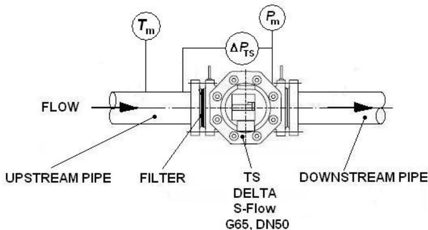
Figure 2 - Recommended installation of the meter
