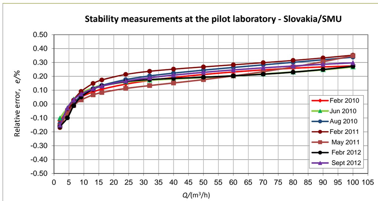
Figure 3 - Stability of the transfer standard
