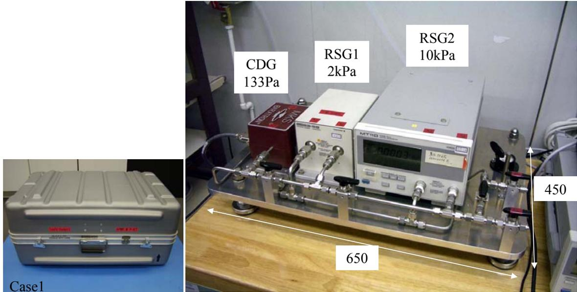
Figure 3.3: Photographs of the pressure transducer part (PTP) and packing case. The three different pressure transducers are mounted on the base-plate.
