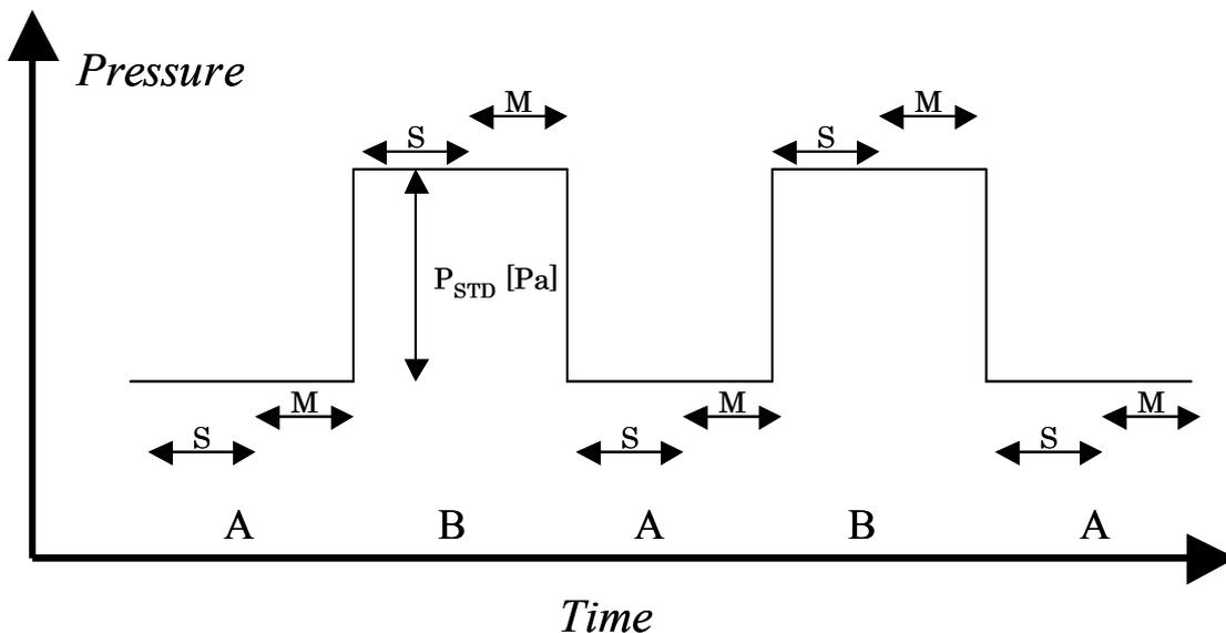
Figure 5.1: Measurement procedure at each pressure point
