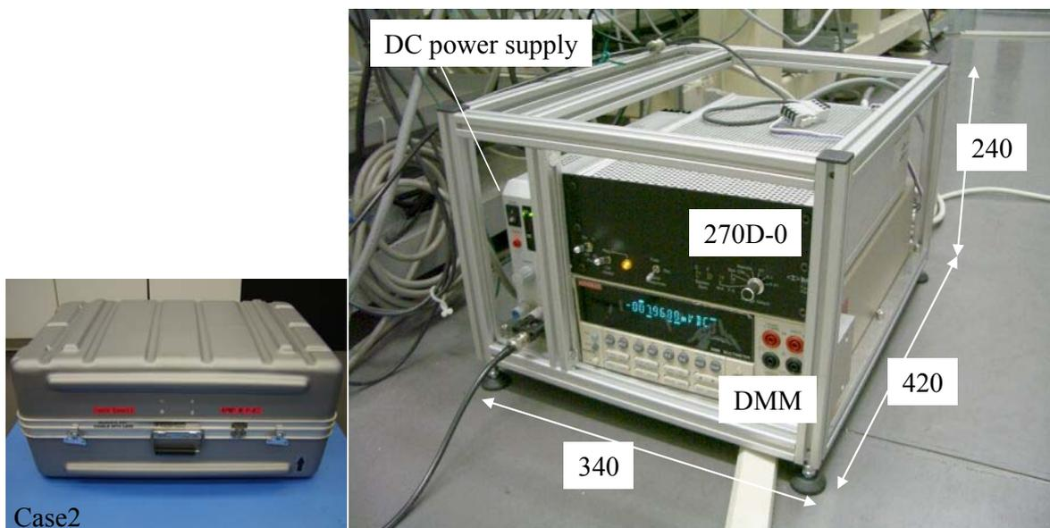
Figure 3.4: Photographs of the support electronics part (SEP) and packing case. The SEP includes a signal conditioner for the CDG, a DMM and a DC power supply within an aluminum mainframe.
