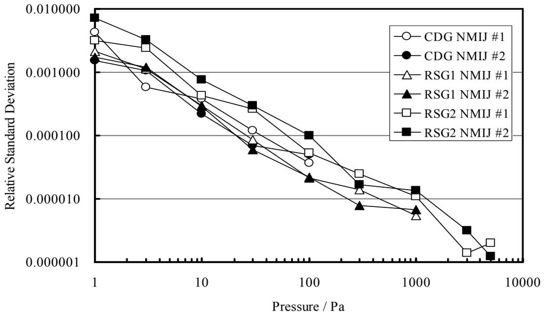
Figure 6.1: The relative standard deviations of the three gauges,  $\sigma(a_{ijk})/a_{ij}$ , where  $\sigma(a_{ijk})$  is the standard deviation of five values of  $a_{ijk}$  about their mean.
