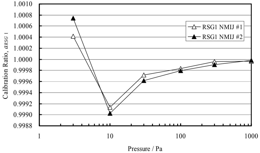
Figure 6.3: Calibration ratios for RSG1 as a function of pressure.
