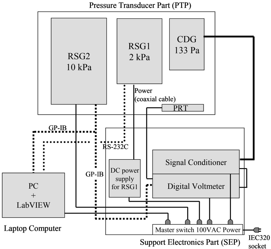
Figure 3.2: Cable interconnections between the pressure transducer part (PTP) and the support electronics part (SEP)
