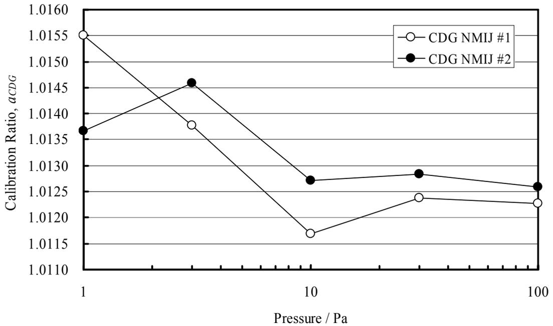
Figure 6.2: Calibration ratios for CDG as a function of pressure.
