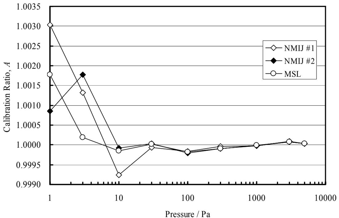
Figure 6.5: Calibration ratios for the transfer standard package after re-scaling as a function of pressure.
