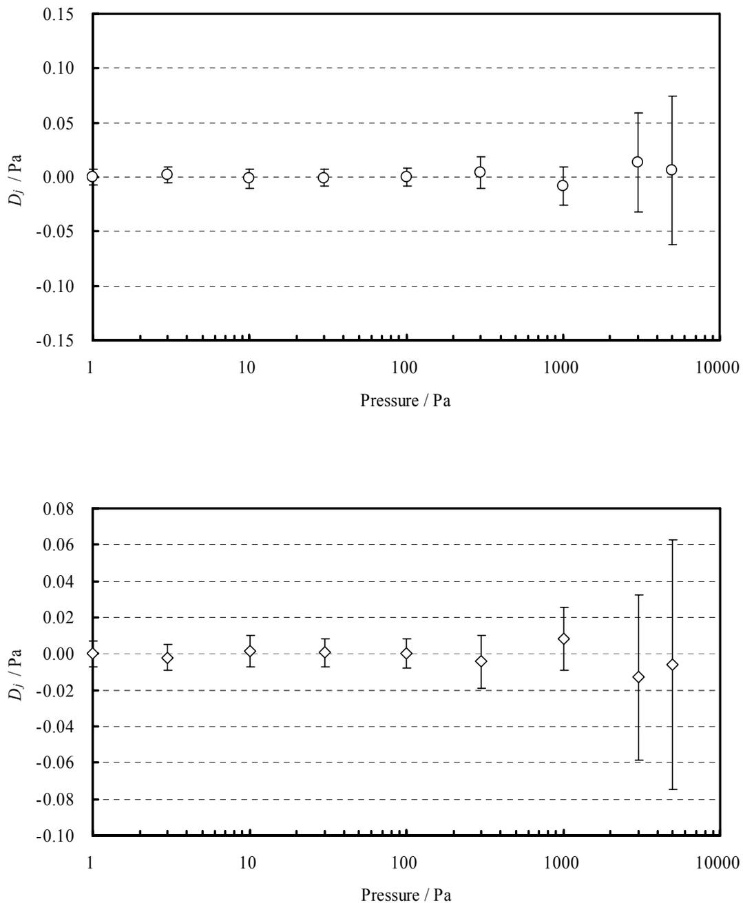
Figure 7.1: Deviations from the APMP KCRVs,  $D_j$ , and the expanded uncertainties of  $D_j$ ,  $U_j$ . The symbols show deviations  $D_j$  and the error bars refer to expanded ( $k = 2$ ) uncertainties  $U_j$ . [Upper] NMIJ/AIST, [Lower] MSL.
