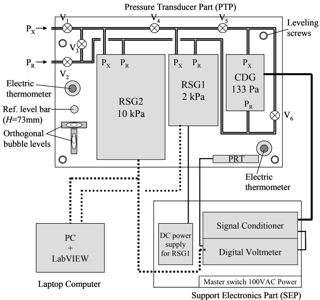
Figure 3.1: Schematic drawing of transfer standard.
