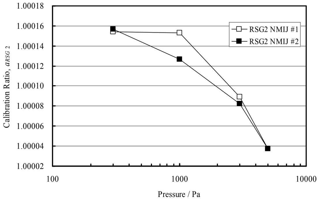
Figure 6.4: Calibration ratios for RSG2 as a function of pressure.
